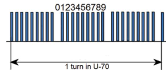
Figure 2.7. Beam structure in the U-70 with injection from the U-3.5
