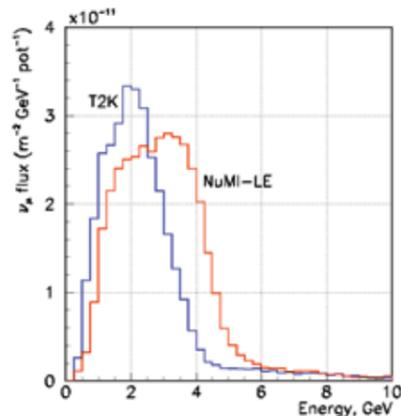
Figure 3.2. The  $\nu_\mu$  beam spectra at the far detector (1160 km) for two variants of the focusing system.
