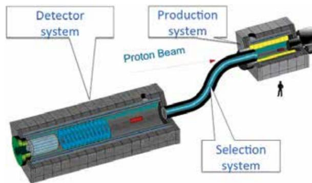
Figure 3.5. 3D view of  $\mu 3in 1$  (Mu3in1) setup.
