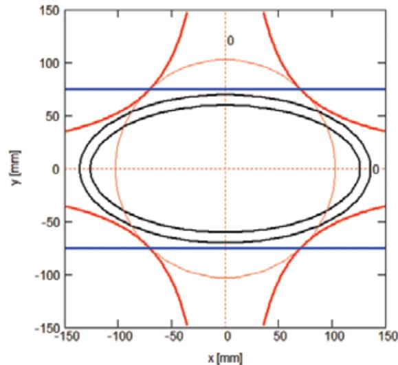
Figure 2.12b. Vacuum chamber and pole surfaces of magnets.
