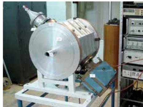
Figure 2.6. "Cold" (radio technical) model of cavity deflector on a test bench
