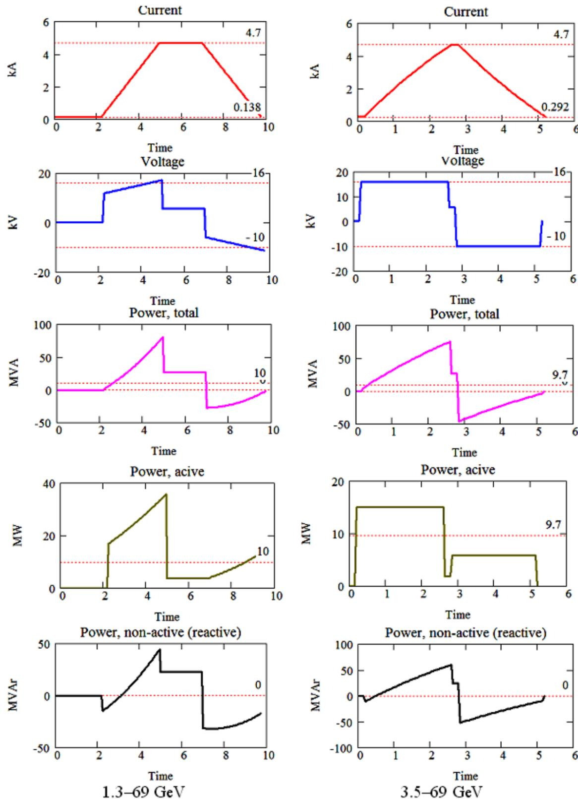
Figure 2.13: Electrical diagrams for a power supply convertor. Peak current is 4.7 kA.
