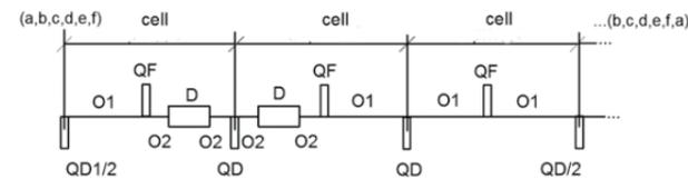
Figure 2.8. Scheme of a half superperiod of the lattice
