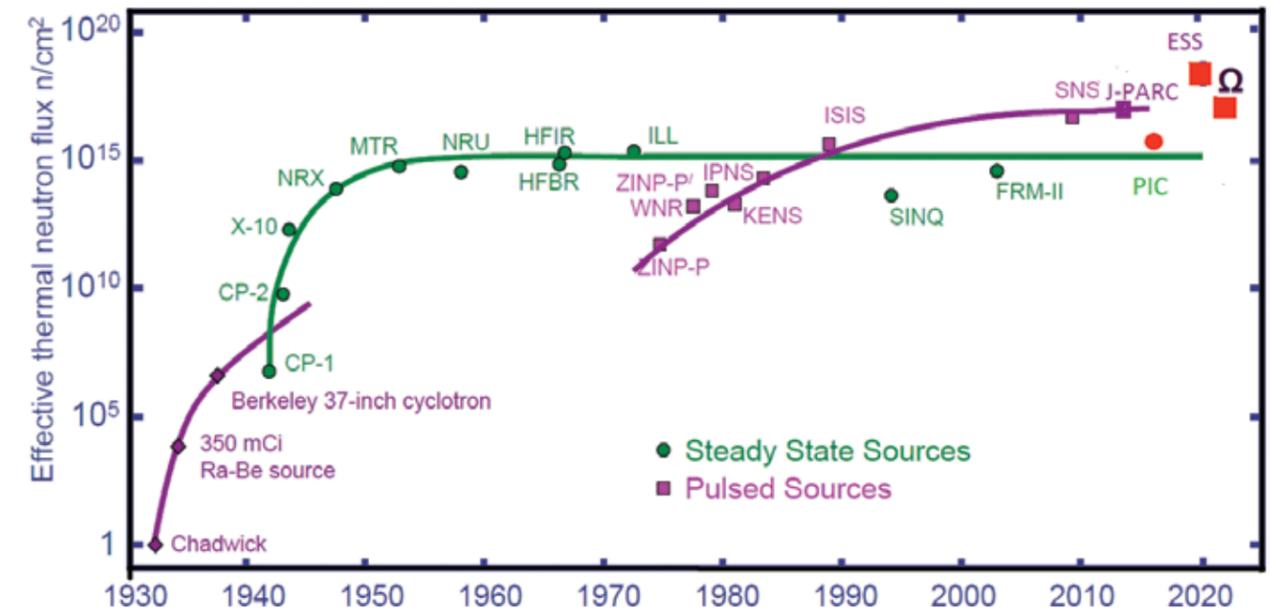
Figure 4.3. Effective thermal neutron flux intensity for different sources (updated from Neutron Scattering, K. Skold and D. L. Price, eds., Academic Press, 1986)
