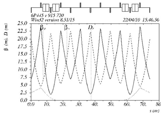
Figure 2.11a. Dynamic functions of magnetic lattice.
