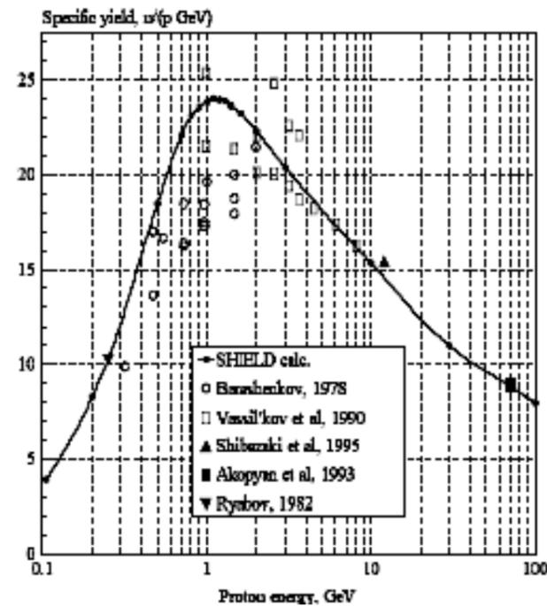
Figure 4.2. Specific yields of neutrons ( $n/p[GeV]$ ) from thick lead target. (from V.S. Barashenkov, EPAN, 9-11, 1978)
