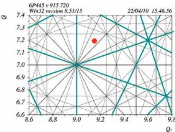
Figure 2.11b. Betatron tune plots and operating point.
