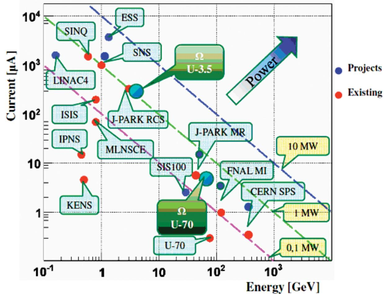
Figure 2. Parameters of high-intensity proton accelerators. Dashed lines mark the levels of definite power. By this parameter, most important for many tasks, the proposed project (RC PS U-3.5) will surpass the existing facilities. Two points are indicated for The OMEGA Project ( $\Omega$ ):
