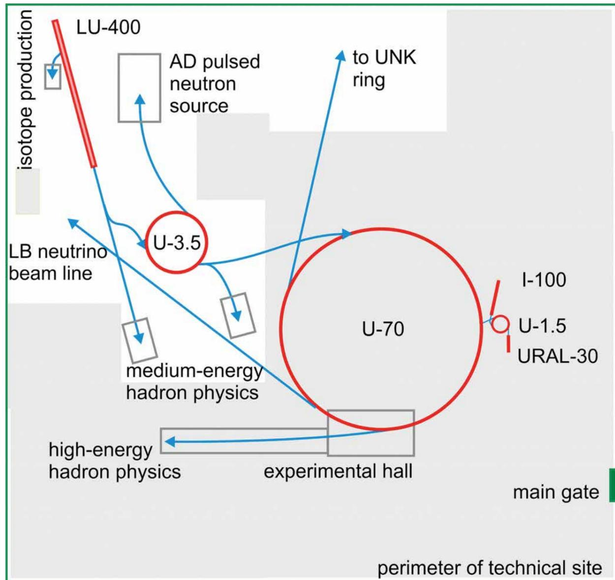
Figure 2.10. Layout of the Facility for Intense Hadron Beams on the IHEP site. Shaded (grey) area shows a zone occupied with the existing civil and engineering infrastructure.
