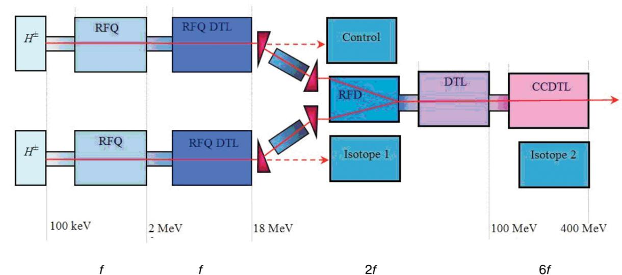
Figure 2.5. Structure of the linear accelerator
