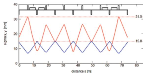
Figure 2.12a. Envelope functions of beam at  $1\sigma$  level
