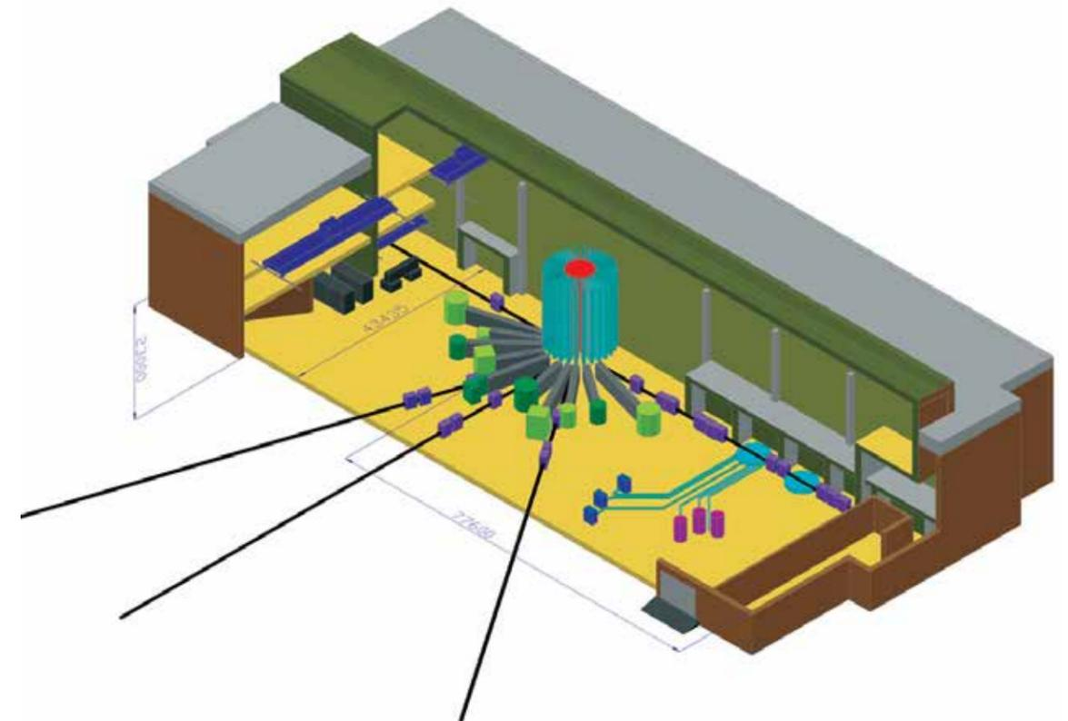
Figure 4.1. Layout of experimental hall with target, system of channels and facilities for experiments with thermal and cold neutrons.
